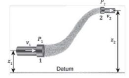
sectional area A, when a pressure force P moves the liquid through a distance  $\Delta x$ , the work performed by the pressure force = the force  $\times$  by the displacement,
