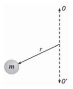
referred to as the second moment of mass, the moment of inertia describes how mass is distributed around an axis.
