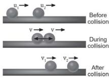
According to Newton's law of collision, the coefficient of restitution (e) can be expressed as follows:
