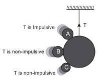
All normal are impulsive but tension T is impulsive only for the ball A
