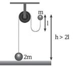
**Sol**. When the lighter ball of mass m is dropped from the initial position, it falls freely for length 2l with the final velocity being v. At this instant, the string gets taut and the velocity of the system becomes v<sub>1</sub> as shown in the figure.
