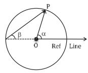
Examine a particle P in motion along a circular path, as depicted in the provided figure. In this scenario, the angular velocity of particle P with respect to both 'O' and 'A' will vary.
