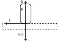
The coefficient of kinetic friction remains unaffected by the relative speed of the surfaces in contact.
