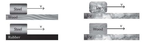
The coefficient of kinetic friction remains unaffected by the surface area in contact. For instance, whether a body rests on its larger or smaller face, the frictional force remains constant.
