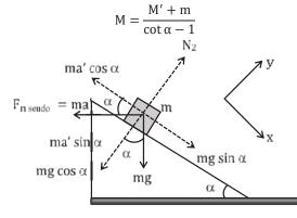
Ex. A particle descends a frictionless inclined plane inclined at an angle  $\theta$  fixed in an elevator ascending with an acceleration  $a_0$ . The base of the incline has a length L. Determine the time taken by the particle to reach the bottom.
