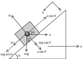
Equating forces in the 'x' direction  $\Sigma \vec{F}_x = m \vec{a}_x \\ mgsin \, \theta = m(a_o - acos \, \theta) \qquad \qquad ... \, (1)$
