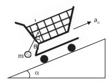
**Sol.** Let's transition into the trolley frame. Since it is a non-inertial frame, we must introduce a pseudo force in a direction perpendicular to the frame's acceleration. Free Body Diagram (FBD) of mass m,
