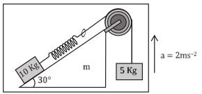
**Sol.** The spring balance gauges the force applied to the spring. In this case, as the spring is considered massless, the measurement corresponds to the tension in the string.
