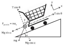
Trolley frame (Non-inertial frame)
