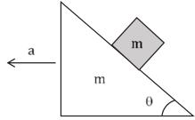
Sol. For the block to fall freely, the normal reaction between the wedge and the block should be zero (N=0). Let's analyze this scenario in a non-inertial (wedge) frame. The components depicted in blue correspond to the weight force, while the components in yellow represent the pseudo force.
