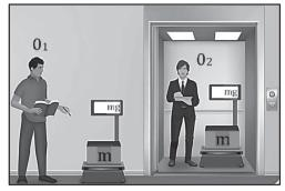
Both observers depict the system using Free Body Diagrams (FBD). The forces exerted on the block include its weight (mg) and the normal reaction (N). Along vertical direction, N=mg
