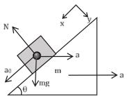
Resolve the components of weight and acceleration along the direction of the inclined surface and perpendicular to it.
