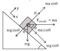
Ex. In the depicted diagram, the measurement on the spring balance (N) can be determined as follows: (Assume  $g = 10 \text{ ms}^{-2}$ ).
