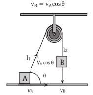
$\begin{aligned} l_1 + l_2 &= 0 \\ -v_A \cos \theta + v_B &= 0 \end{aligned}$
