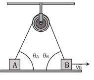
**Sol.** In this scenario, block B moves to the right. Consider the velocity component along the length of the string at both ends.
