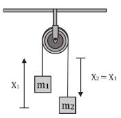
Examine the magnitude of displacement for two objects. According to the inextensibility constraint of the string,  $x_1=x_2$
