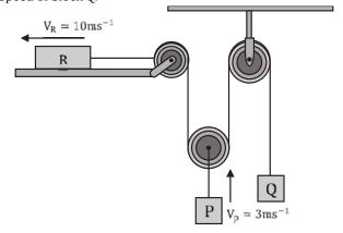
**Sol.** In this scenario, the direction of motion for block Q is uncertain. For the purpose of analysis, we presume that the block is ascending. If this assumption proves incorrect, a negative sign in the velocity result would indicate that the block is moving in the opposite direction to what was initially assumed. Therefore, we assume that block Q moves upward concurrently with the leftward motion of block R.
