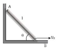
Sol. As end B moves towards the right, end A will move downwards, and both ends will consistently stay in contact with the surface. Adopt the specified velocity variables and coordinate axes. Assume the coordinates of point B as (x,0) and the coordinates of point A as (0,y). In triangle,
