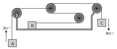
**Sol.** In the provided system, there are three mobile objects and one movable pulley. Assume the acceleration of block B as 'a' in the right direction. Segment each string into intercepts and formulate the constraint equations for them. Three equations are required for the three objects. Consider the acceleration as a variable for both the pulley and the blocks, as illustrated.
