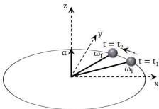
It is the limit of average angular acceleration as  $\Delta t$  approaches zero i.e.
