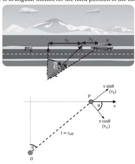
Take parallel and perpendicular components of the linear velocity V.
