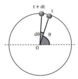
Instantaneous Angular Velocity refers to the immediate speed at which the angular position changes at any given moment in time.
