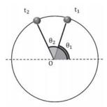
If  $\theta_1$  and  $\theta_2$  are the angular positions at time  $t_1$  and  $t_2$  respectively, then
