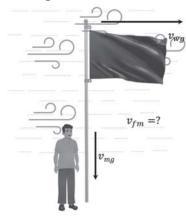
When the man is at rest, the velocity of the flag is same as the velocity of the wind, i.e.  $\vec{v}_{fg} = \vec{v}_{wg}$
