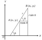
Consider the line segment connecting the points, which has a length of r, and let the line be oriented at an angle  $\theta$  relative to the x-axis.
