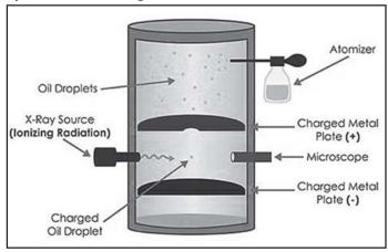
An oil droplet descends through a hole in the upper plate, and the air between the plates is exposed to X-rays, causing the ejection of electrons from air molecules. Some of these electrons are captured by the oil droplet, imparting a negative charge to it.
