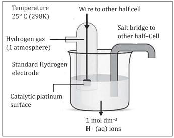
The surface of platinized platinum exhibits a notably high adsorption activity. Consequently, it is imperative to shield this surface from atmospheric oxygen and organic substances. Catalyst deactivation or poisoning can occur in the presence of substances like arsenic and sulfur compounds.
