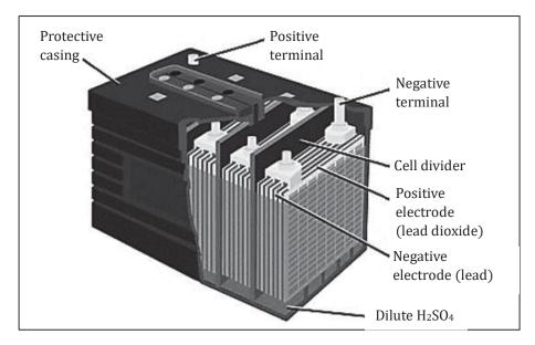
Each battery consists of a number of voltaic cells connected in series. Three to six such cells are generally combined to get 6-to-12-volt battery.
