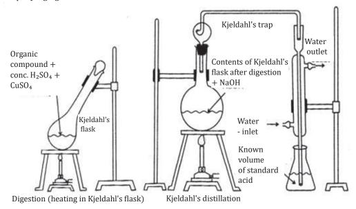
In this method, a known mass of the organic compound undergoes digestion with concentrated  $H_2SO_4$  in the presence of potassium sulfate and a small amount of copper sulfate within an elongated-neck flask. The nitrogen present in the compound undergoes quantitative conversion into ammonium sulfate through the chemical reaction:
