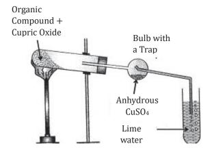
This process is commonly referred to as the copper oxide test.
