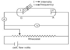
Here the plate (1) is called emitter or cathode and other plate (2) is called collector or anode.
