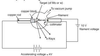
The melting point, specific heat capacity and atomic number of target should be high. When voltage is applied across the filament then filament on being heated emits electrons from it. Now for giving the beam shape of electrons, collimator is used. Now when electron strikes the target then x-rays are produced.
