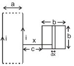
Let current i flow in the loop having  $\infty$ -by long sides. Consider a segment of width dx at a distance x as shown flux through the regent
