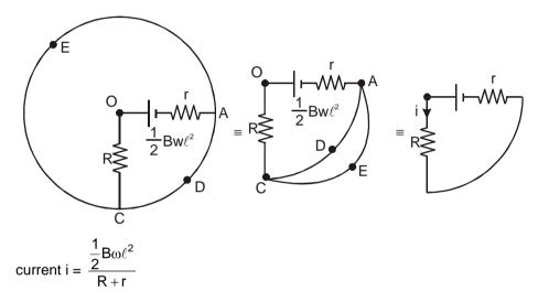
**Example 14.** Solve the above question if the length of rod is 2L and resistance 2r and it is rotating about its centre. Both ends of the rod now touch the conducting ring
