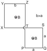
Solution :Induced emf in part PQST =  $\beta a^2$  (in anticlockwise direction, from Lenz's Law)Similarly Induced emf in part TXYZ =  $\beta b^2$  (in anticlockwise direction, from Lenz's Law)Total resistance of the part PQST = $\lambda$ 4a.Total resistance of the part TXYZ =  $\lambda$ 4b. The equivalent circuit is as shown in the following diagram.
