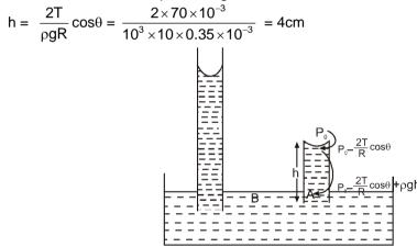
Now suppose we use shorter capillary of same radius, but its length is only 2 cm. It is slightly dipped in the water.
