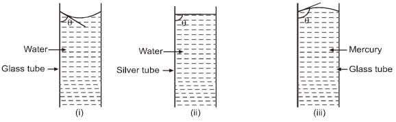
If we fill water in glass tube, the surface becomes concave in shape, if water is filled in silver tube, the surface becomes horizontal and if Hg is filled in glass tube, the surface becomes convex.
