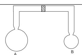
Solution : Radius of curvature of smaller bubble 'B' is less so pressure inside the smaller bubble will be more  $\left(P_0 + \frac{4T}{r}\right)$ . Air will flow from high pressure to low pressure, so it will flow from smaller
