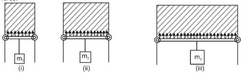
Consider three cases (i), (ii) and (iii). In which case, the surface tension force on the slider is more? Practically it is observed that in case (i) surface tension force on slider is least, it is more in case (ii) and most in case (iii). In case (iii), we have to hang more weight to keep the slider in equilibrium. From this example it is clear that surface tension force depends on contact length which is greatest in case (iii)
