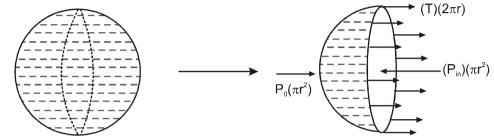
(i) Pushing force on the left half liquid due to right half liquid will be  $(P_{in})(\pi r^2)$
