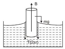
(i) buoyancive force of water acting upward
