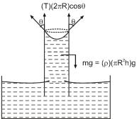
As we dip the capillary in water, the surface pulls the capillary walls in downwards direction, so the capillary walls pulls the surface in upward direction as shown in figure, due to which water will rise up till the forces get balanced.
