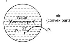
Generally we can say that pressure at concave part will be greater than pressure at convex part by  $\frac{21}{r}$  where r is radius of curvature of the surface between them.
