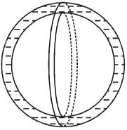
**Solution :** The bubble also have two surfaces: the inner surface and the outer surface. And in the small thickness between them, there is some liquid. So the surface tension force will be applied by inner surface as well as the outer surface  $[T(2\pi R)]$ .
