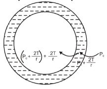
So pressure inside the liquid bubble =  $P_0 + \frac{4T}{r}$
