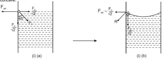
**Case -II** : If water is filled in silver tube,  $F_{ad} = \frac{F_c}{\sqrt{2}}$  so resultant will be vertically downwards. So liquid
