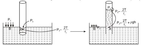
If we dip the capillary tube in water, due to the concave surface, pressure just below the surface becomes  $P_0 - \frac{2T}{r_c}$ , while on the other points at the same horizontal level, pressure is  $P_0$ . Due to this less pressure
