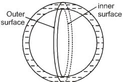
**Example 5.** A thin disc of radius R, just touching the liquid surface, forms one arm of a balance. The plate is balanced by some weight on the other side of the balance. How much extra weight should be added on the other side, so that the disc can just come out of water ?
