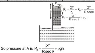
**Example 12.** A small air bubble (cavity of air) of radius r is at depth 'h' .Find the pressure inside the bubble.
