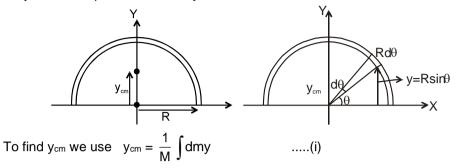
Here for dm we consider an elemental arc of the ring at an angle  $\theta$  from the x-direction of angular width d $\theta$ . If radius of the ring is R then its y coordinate will be R sin $\theta$ , here dm is given as
