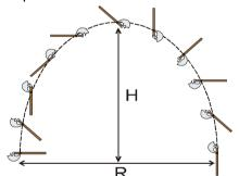
The motion of axe is complicated but the COM is moving in a parabolic motion.
