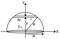
The mass dm of this disc can be given as dm =  $\frac{3M}{2\pi R^3} \times \pi r^2 dy = \frac{3M}{2R^3} (R^2 - y^2) dy$
