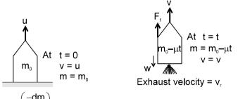
Further, let  $\left(\frac{-dm}{dt}\right)$  be the mass of the gas ejected per unit time and  $v_r$  the exhaust velocity of the
