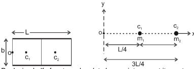
Replacing half of rectangular plate by a point mass at its center of mass as shown in figure.
