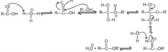
If we follow the forward reactions in this mechanism, we have the mechanism for the acid catalysed esterification of an acid. If however, we follow the reverse reactions, we have the mechanism for the acid catalysed hydrolysis of an ester.
