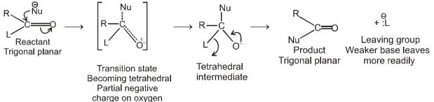
The tetrahedral intermediate formed when a nucleophile attacks the carbonyl carbon of a carboxylic acid derivative is not stable and cannot be isolated.
