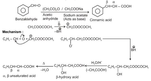
**Note :** By knowing  $\alpha$ ,  $\beta$ -unsaturated acid we can get idea about the anhydride used in perkin reaction. This can be done by keeping 'H' at  $\alpha$  and –OH at  $\beta$ -carbon atom followed by breaking  $\alpha$ ,  $\beta$  carbon. By this we can know about acid and it will be anhydride of this acid only.
