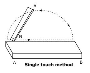
By Stroking the iron piece with the north pole of the bar magnet, end A becomes the north pole and end B the south pole.
