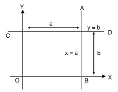
Similarly, the equation of the straight line CD parallel to the X-axis and at a distance 'b' from it is y = b. By putting b = 0 we deduce that the equation to the X-axis is y = 0
