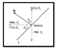
Net force along the vertical direction is zero since there is no acceleration along this direction.
