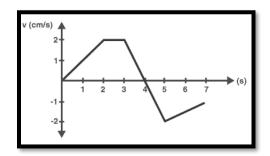
Consider the velocity-time graph shown above. Here, between the time intervals of 0-2 seconds, the velocity of the particle is increasing with respect to time; hence the body is experiencing a positive acceleration as the slope of the v-t curve in this time interval is positive.
