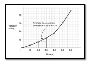
Average acceleration: In the velocity-time graph shown above, the slope of the line between the time interval  $t_1$  and  $t_2$  gives the average value for the rate of change of velocity for the object during the time  $t_1$  and  $t_2$ .
