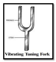
**2.** Take a tuning fork. Hold it from its stem and strike it with a rubber pad or hammer. You will observe that the prongs of the tuning fork vibrate and at the same time sound is produced (Figure).
