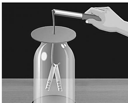
Fig. A simple electroscope
