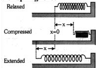
The potential energy of an ideal spring associated with a spring force when compressed or elongated by a distance x from its natural is given by the following expression  $U = \frac{1}{2}kx^2$ .
