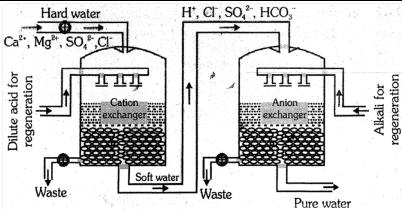
This water becomes soften but not used for drinking purpose because this water contain the impurity of acid. To remove anion of hardness this acidic water then passed through another bed containing anion exchanger. This exchanger removes anion like  $Cl^-$ ,  $SO_4^{-2}$  &  $HCO^{3-}$ .
