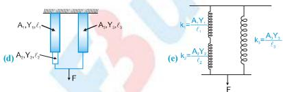
**Ex.** A mass 'm' is attached with rods as shown in figure. This mass is slightly stretched and released whether the motion of mass is S.H.M., if yes then find out the time period.
