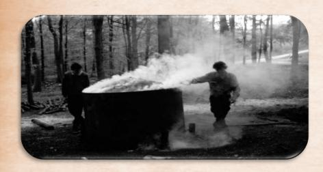
This had several problems: charcoal was too fragile to transport across long distances: its impurities produced poorquality iron: it was in short supply because forests had been destroyed for timber: and it could not generate high temperatures.
