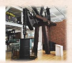
Another steam engine was built by Thomas Newcomen (1663-1729) in 1712. This had the major defect of losing energy due to continuous cooling of the condensing cylinder.
