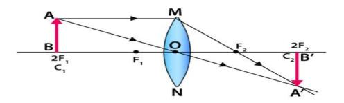
• When an object is placed in between the center of curvature and focus, the real image is formed behind the center of curvature. The size of the image is larger than that of the object.
