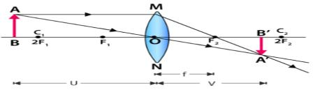
• When an object is at the center of curvature, the real image is formed at the other center of curvature. The size of the image is the same as compared to that of the object.
