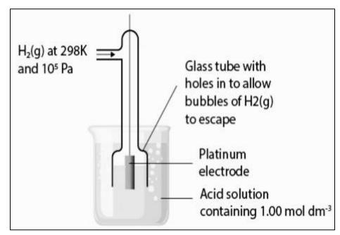
Electrodes potentials vary with temperature and so a standard temperature is defined. This is 298K. Altering the concentration of any ions appearing in the half-reactions also affects the voltages, so a standard concentration of 1.00 mol dm<sup>-3</sup> is chosen. Standard pressure is 10<sup>5</sup>Pa.The potential of a standard hydrogen half-cell is defined as 0.0V a value chosen for convenience.
