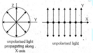
The resultant electromagnetic: wave is a superposition of waves produced by the individual atomic sources and it is called unpolatised light. In ordinary or unpolarised light, the vibrations of the electric vector occur symmetrically in all possible directions in a plane perpendicular to the direction of propagation of light.
