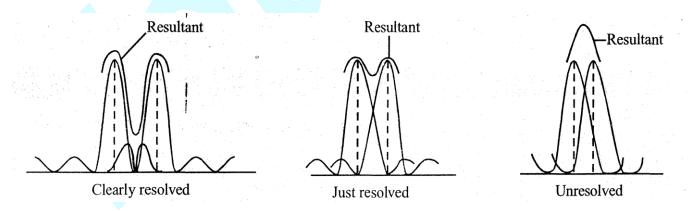
Two points are just resolved by an optical system when the central maximum of the diffraction pattern due to one falls on the first minimum of the diffraction pattern of the other.
