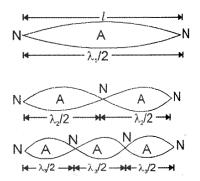
Similarly, if the wire vibrates in three segments (fig.) and the wavelength in this case be  $\lambda_3$ , then
