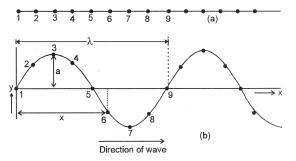
As the wave reaches the particles beyond the particle 1, the particles start oscillating. If the speed of the wave be v, then it will reach particles 6, distance x from the particle 1, in x/v sec. Therefore,
