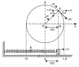
Suppose the particle is on the top of the circle (Y-axis) at t = 0. The radius OP make an angle  $\theta$  =  $\omega$ t with the Y-axis at time t. Drop a perpendicular PQ on X-axis. The components of position vector, velocity vector and acceleration vector at time t on the X-axis are
