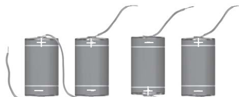
Connecting two cells together to make a battery
