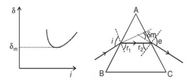
Theoretical analysis and experimental observations converge to reveal that the angle of deviation  $\delta$  attains its minimum value when the trajectory of the light ray passing through the prism exhibits symmetry.
