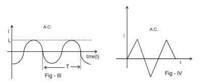
This AC current repeats its values after specific time intervals, known as the time period. The angular frequency  $\omega$  is equal to  $2\pi$  times the frequency 'f,' where  $\omega = 2\pi f$ .
