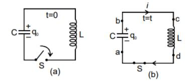
We will proceed to formulate an equation that describes the oscillatory behavior of charge and current within an L-C (inductor-capacitor) circuit. Please consult the provided figure for reference.
