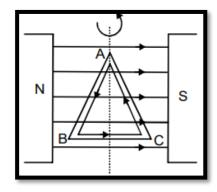
Now, the couple on a current-carrying coil in a magnetic field is given by  $\tau = MB \sin \theta$  since the plane of the coil is parallel to the magnetic field, the angle between M and  $\vec{B}$  will
