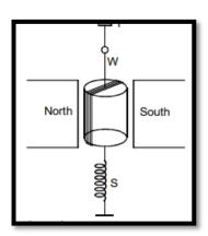
The current to be measured is passed through the galvanometer. As the coil is in the magnetic field  $\vec{B}$  of the permanent magnet, a torque  $\vec{I} = ni\vec{A} \times \vec{B}$  acts on the coil. Here n = ni number of turns, i = ni current in the coil  $\vec{A} = ni$  area-vector of the coil and  $\vec{B} = ni$  magnetic field at the site of the coil. This torque deflects the coil from its equilibrium position.
