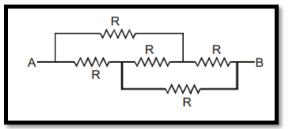
**Sol.** This arrangement can be modified as shown in figure since it is balanced wheat stone bridge.
