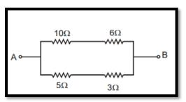
**Ex.** Find the equivalent resistance between A and B
