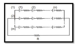
Total number of cells in the combination = mn. As e.m.f. of each row = nE and all the rows are connected in parallel, hence net e.m.f of battery = nE. Internal resistance of each row = nr. As m such rows are connected in parallel, hence total internal resistance of battery =  $\left(\frac{nr}{m}\right)$
