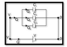
**Example.** Three initially uncharged capacitors are connected to a battery of 10 V is parallel combination find out following
