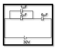
**Solution:** It can be simplified as  $C_{eq} = \frac{18}{9} = 2\mu F$
