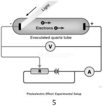
In the experimental setup, two plates, denoted as C and D, are integrated into a circuit connected to a battery (B) and an ammeter (A). Plate D, exposed to radiation through a quartz window (W), experiences the emission of electrons, resulting in the flow of current in the circuit. This electric current generated by the ejection of electrons is termed photocurrent. Additionally, plate C has the capability to be adjusted to a desired potential, either positive or negative, in relation to plate D.
