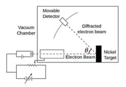
The electron gun utilized in the experiment comprises a Tungsten filament, which emits electrons through thermionic emission, a process in which electrons are released when the filament is heated to a specific temperature. The experimental setup also incorporates an electrostatic particle accelerator, consisting of two plates with opposite charges (positive and negative), employed to accelerate the electrons to a known potential.
