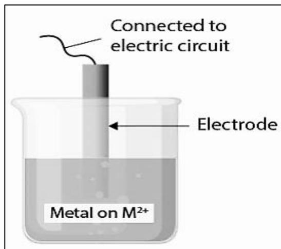
If the oxidation takes place at the electrode, it is called the oxidation potential
