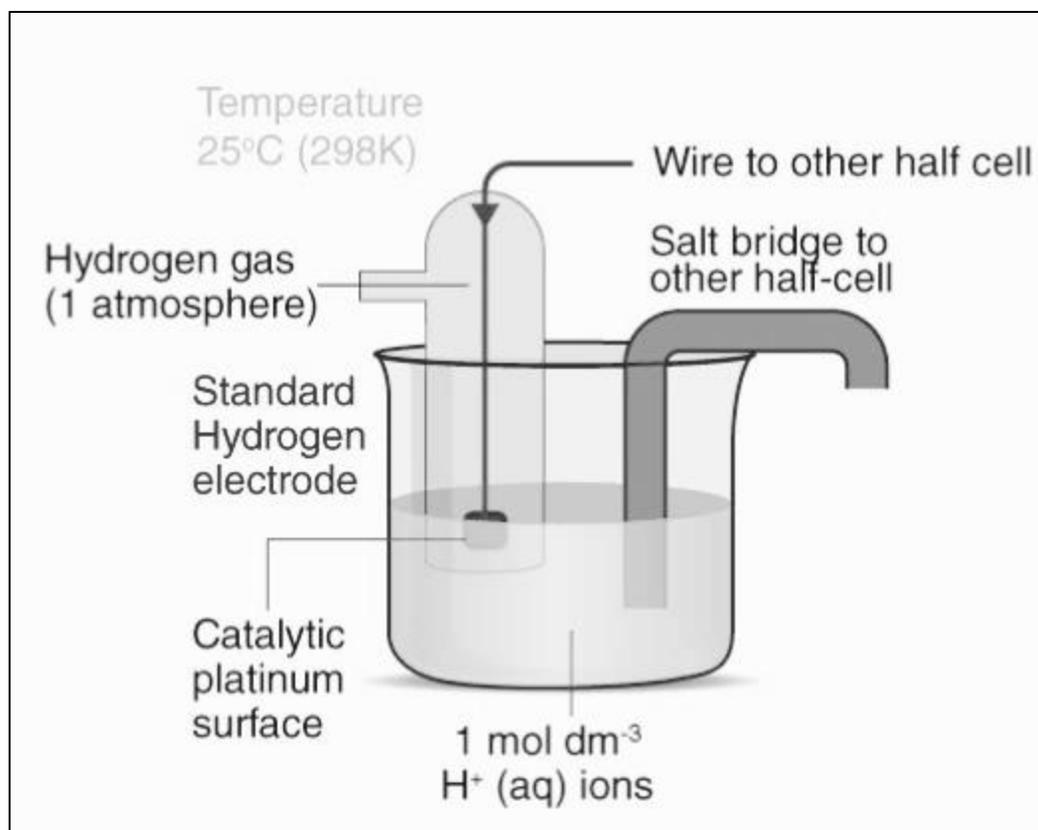
The platinized platinum surface has a very high adsorption activity. Therefore, this surface must be protected from atmospheric oxygen as well as from organic substances. Substances such as arsenic and sulphur compounds can deactivate or poison the catalyst.
