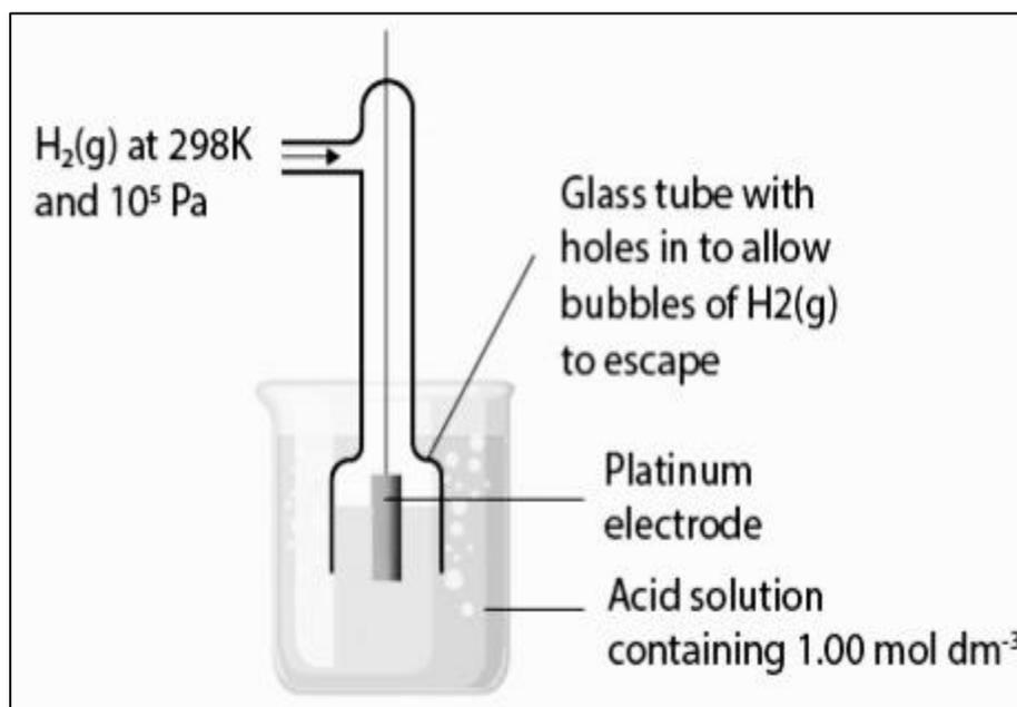
Electrodes potentials vary with temperature and so a standard temperature is defined. This is 298K. Altering the concentration of any ions appearing in the half-reactions also affects the voltages, so a standard concentration of  $1.00 \text{ mol dm}^{-3}$  is chosen. Standard pressure is  $10^5 \text{ Pa}$ . The potential of a standard hydrogen half-cell is defined as  $0.0 \text{ V}$  a value chosen for convenience.
