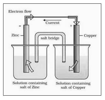
These reactions occur in two different portions of the Daniel cell. The reduction half-reaction occurs on the copper electrode while the oxidation half-reaction occurs on the zinc electrode. These two portions of the cell are also called half-cells or redox couples. The copper electrode may be called the reduction half-cell and the zinc electrode, the oxidation half-cell.
